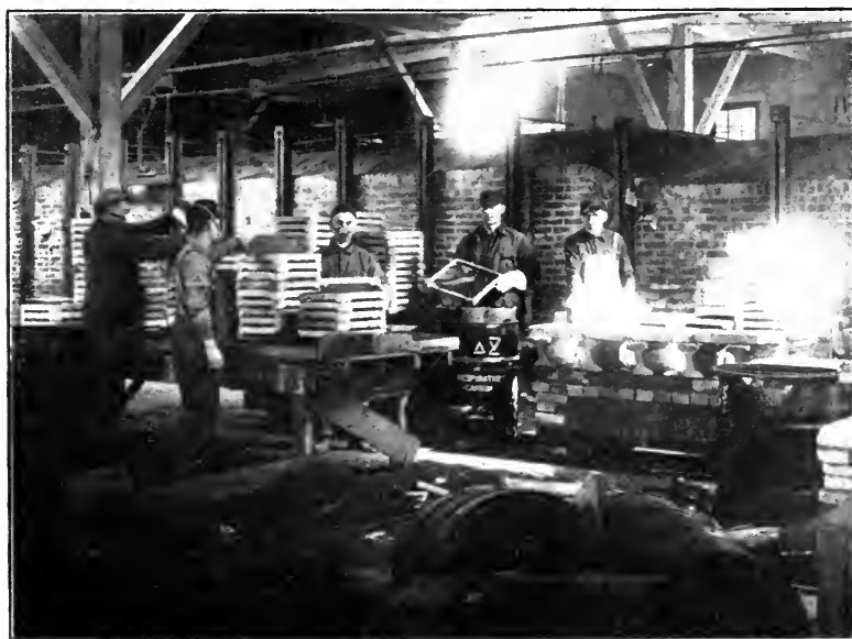
The Tunnel Kiln Furnace Shifts Unloading Respirator Carbon, Filling and Striking Trays and loading Crude Carbon
